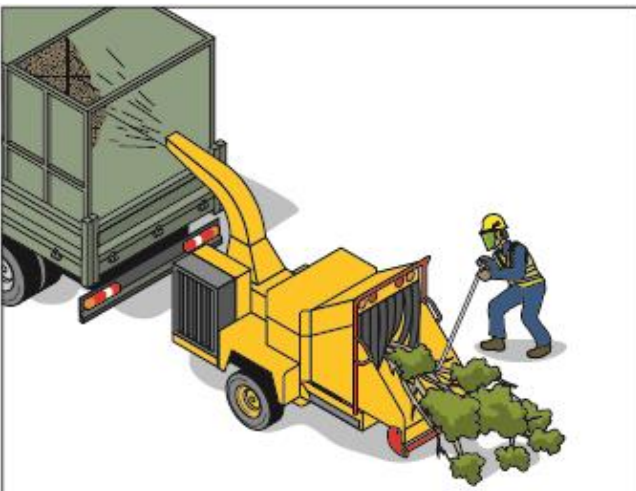
Figure 4 Using a push-stick to feed shorter branches into a woodchipper
