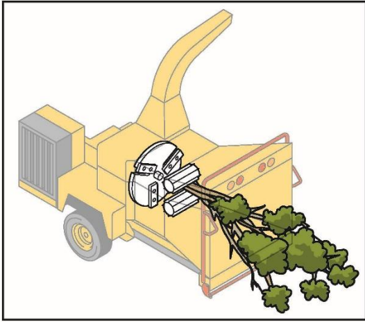
Figure 5 Disc-type woodchipper showing in-feed rollers and cutting disc
