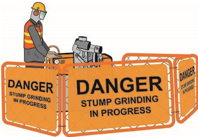
Figure 8 Protective barriers separating people from stump grinding operations.
